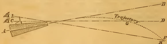
A B , line of fire. C D , natural line of sight. E F , artificial line of sight. G , point-blank. H , artificial point-blank.
